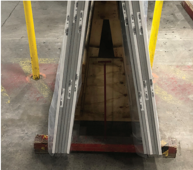
Figure C-1: Safety Devices (safety posts and safety support)
